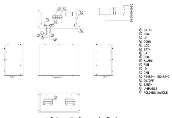
▲ Schematic diagram for Rack type
